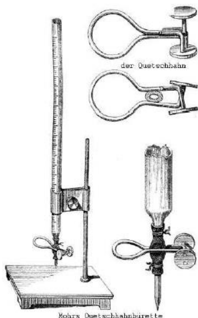
Figure 1: Mohr's pinch cock burette ["Meyers Konversations-Lexikon" [Meyers Conversational Dictionary] 1885–1890, 4th edition]
